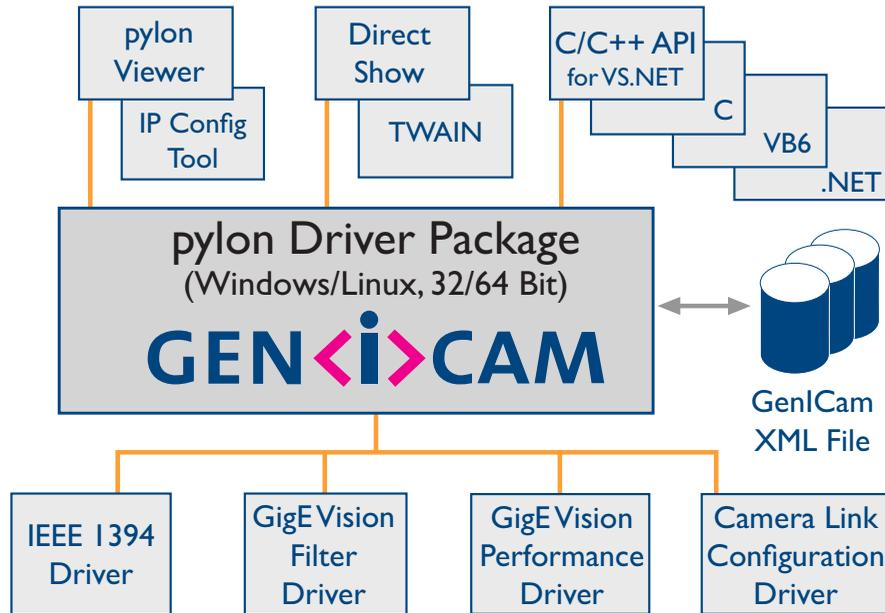
The internal architecture of the pylon driver package is based on GenICam Technology, which offers you easy access to the newest camera models and the latest features. Changes to an existing camera device in your application essentially become a plug-and-play process.
