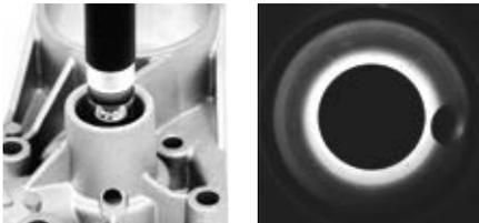
Inspection of holed parts of an engine.
