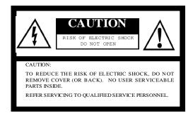
The lightning flash with arrowhead symbol, within an equilateral triangle, is intended to alert the user to the presence of uninsulated "dangerous voltage" within the product's enclosure that may be of sufficient magnitude to constitute a risk of electric shock to persons.
