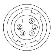
Note 1: Trigger input signal can be assigned either on Camera Link connector (CC1) or on the No. 2 pin of the interface connector through the camera setting communication.
